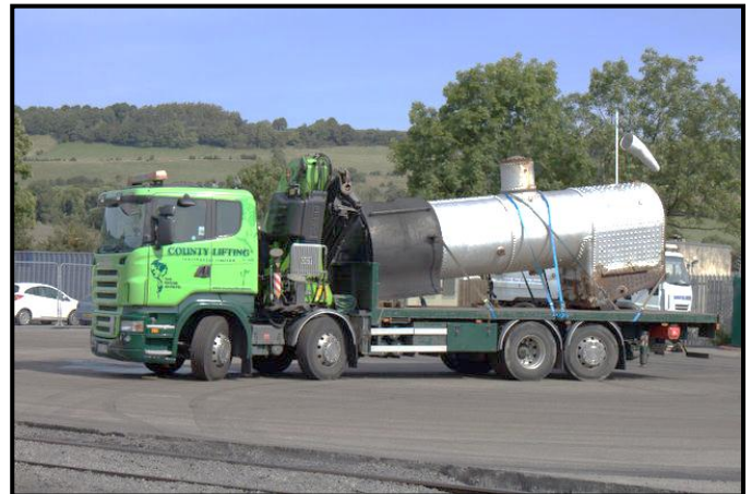
September 3 rd in Wolsingham depot. The boiler of No 40 is lifted from the frames and loaded on to the truck transport to Loughborough Locomotive Works. (Photos : Left : Keith McNally, right : Richard Maughan)
