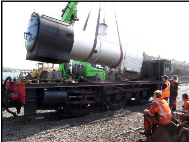
September 3 rd in Wolsingham depot. The boiler of No 40 is lifted from the frames and loaded on to the truck transport to Loughborough Locomotive Works. (Photos : Left : Keith McNally, right : Richard Maughan)
