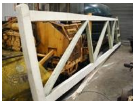
Partially completed crossing gate, this is the shorter one ( Photo : David Scott )
