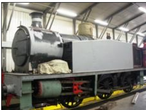
No 40 : tanks and cabsides in place 11 March ( D Scott)
