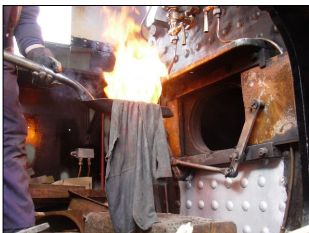
Lighting the fire for the low pressure steam test
