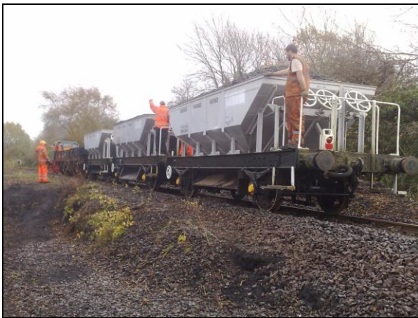
The WRT 'Dogfish' wagons being put to use at the work location at Broken Banks in November ( A Gregory )
