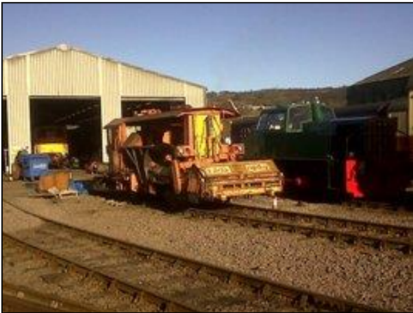
The Ballast Regulator ready for action in Wolsingham Yard
