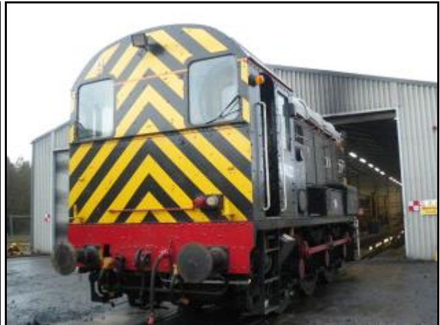
Shunter 08622 outside the Depot where it is undergoing traction motor replacement prior to returning to Teesport as part of BARS lease fleet (Both photos : D Scott)
