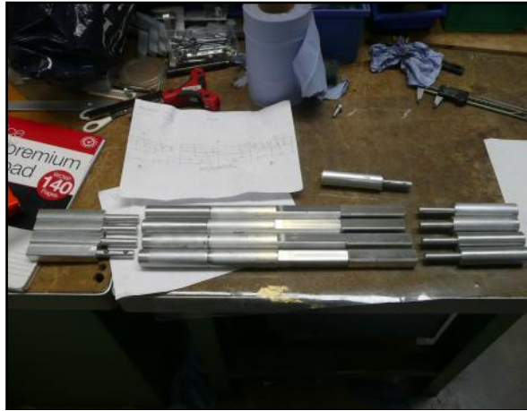
The new train staffs in the course of manufacture
