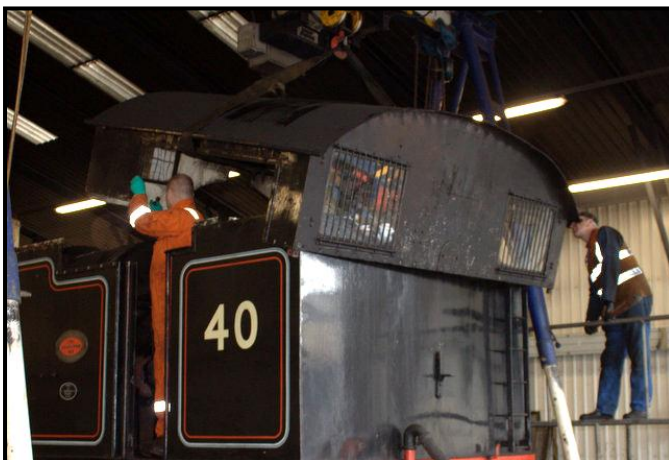
Four stages in the dismantling of No 40, prior to accessing the boiler so that it can be moved to the boiler-smiths for refurbishment. Starting at top left, the side tanks are removed, then the cab sides followed by the cabroof. Last Photo (Bottom right) shows the loco ready to lift the boiler. Photo : David Scott, all other photos : Richard Maughan.
