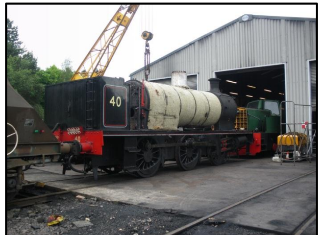
Four stages in the dismantling of No 40, prior to accessing the boiler so that it can be moved to the boiler-smiths for refurbishment. Starting at top left, the side tanks are removed, then the cab sides followed by the cabroof. Last Photo (Bottom right) shows the loco ready to lift the boiler. Photo : David Scott, all other photos : Richard Maughan.
