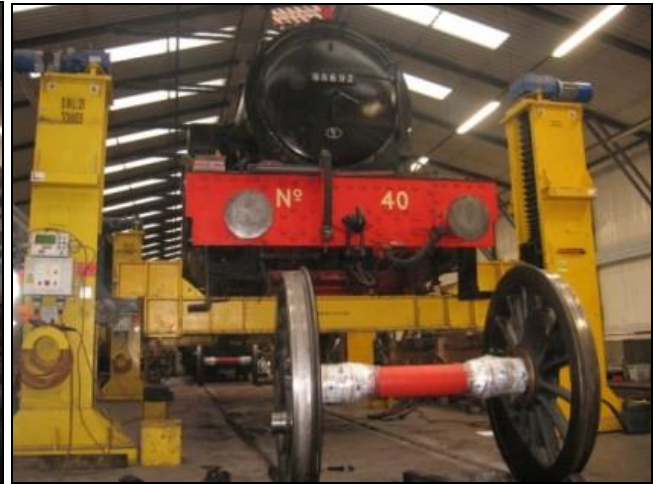
No 40 with one of the two re-machined axles ( Both photos : Norman Swindle )
