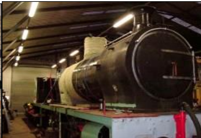
No 40 in Wolsingham depot, boiler back in the frames and restoration work underway
